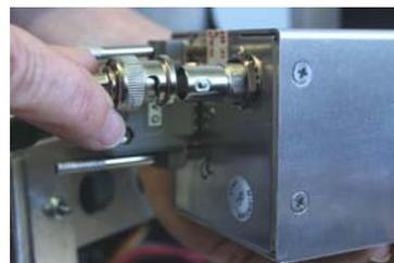
Present the M760 to the rear face of this hole. The stepped round face will insert through the hole, and should appear flush with the front of the instrument panel when correctly positioned. Rotate the M760 to align the four M4 machine screws.
